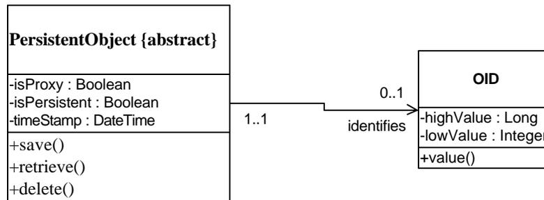
**Figure 6. The design of PersistentObject and OID.**
